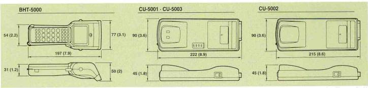
Dimeters are in millimeters (inch)
