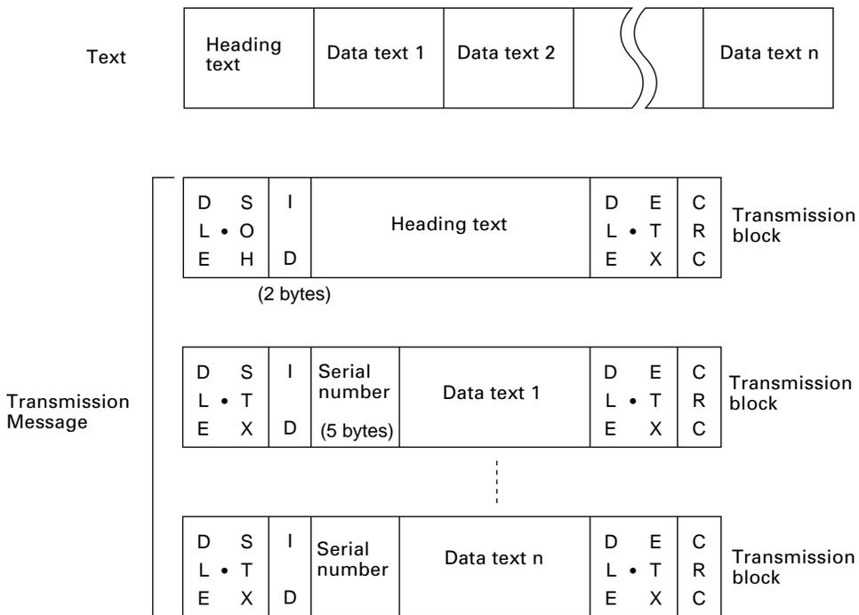
In the above figure, DLE SOH, DLE STX and DLE ETX are text control characters as described in [ 2 ] Control Characters, (2). An ID denotes the ID number of the receiver station, expressed by two bytes. A serial number is expressed by a five-digit decimal number, starting from 00001 to 32767, and identifies data texts. For the CRC-16, refer to Appendix B, B.2, "BHT-Ir protocol, " [ 3 ].
