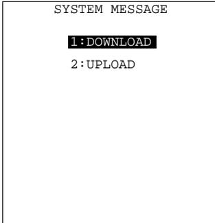
Pressing the **[6]** key while holding down the **[SF]** key on the SYSTEM MENU calls up the screen shown at left.
