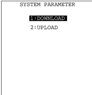
Pressing the **[3]** key while holding down the **[SF]** key on the SYSTEM MENU calls up the screen shown at left.
