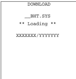
While the downloading operation is in progress, the screen shown at left is displayed indicating the file name and the number of received records/the total number of records.
