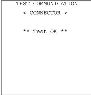
Upon normal completion of the test, the BHT beeps once and shows the screen at left.
