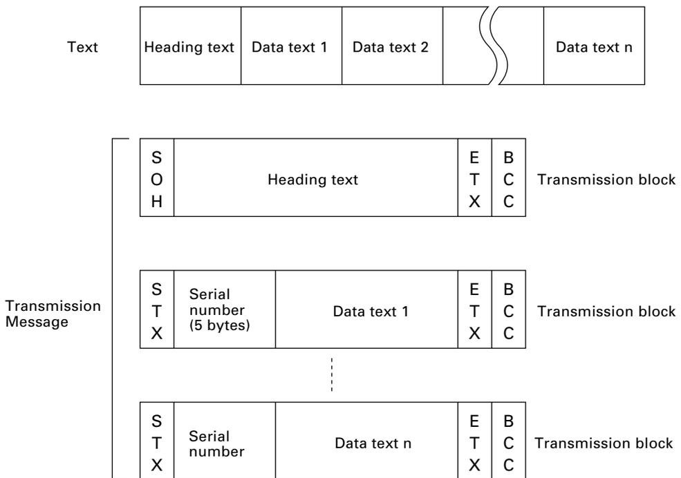
In the above figure, SOH, STX, and ETX are text control characters as described in [ 2 ] Control Characters, (2). A serial number is expressed by a five-digit decimal number, starting from 00001 to 32767, and identifies transmitted data texts. For the BCC, refer to Appendix B, B.1, "BHT-protocol," [ 3 ].
