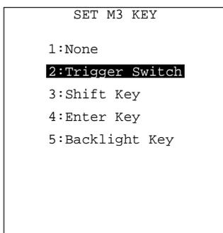
Selecting the "2:M1 KEY," "3:M2 KEY," "4:M3 KEY" or "5:M4 KEY" on the SET KEY menu calls up the screen as shown at left. (This example appears when the "4:M3 KEY" is selected.)
