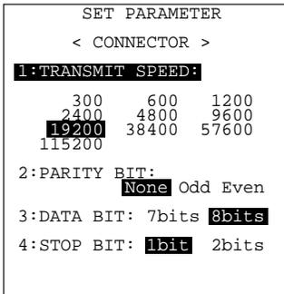
Selecting "1:PARAMETER" on the SET CONNECTOR screen calls up the screen shown at left.
