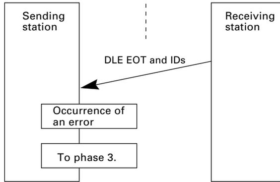
■ **Phase 2 with iterated transmission of DLE ENQ and IDs due to no response or invalid response**
