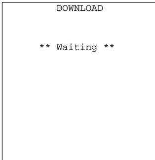
Selecting "1:DOWNLOAD" on the SYSTEM PARAMETER transfer menu calls up the screen shown at left. With this screen displayed, the BHT waits for the BHT system parameter file to be downloaded.
