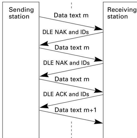
If the sending station receives a sequence of DLE NAK and IDs 10 times in succession or it fails to send a same transmission block, it shifts to phase 3 to terminate the message transmission abnormally. Even if phase 3 terminates normally, the transmission results in an abnormal end.
