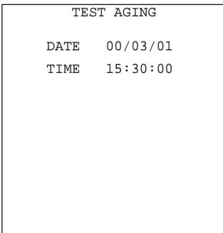
Selecting "4:AGING" on the TEST menu proceeds to the aging test while showing the current date and time on the LCD. (This test is intended for personnel which check the BHT in the factory.)
