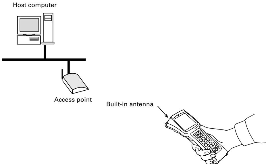
For data transfer using radio link, it is necessary to configure a wireless local area network (wireless LAN) connecting the BHT-7500S and access points.
