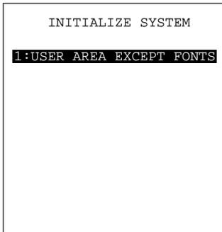
Press the **PW** key while holding down the **SF**, **M1** and **0** keys together.
