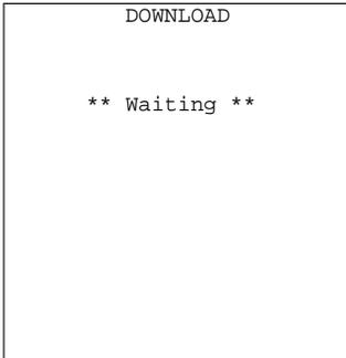
Selecting "1:DOWNLOAD" on the SYSTEM MESSAGE transfer menu calls up the screen shown at left. With this screen displayed, the BHT waits for the system message file to be downloaded.
