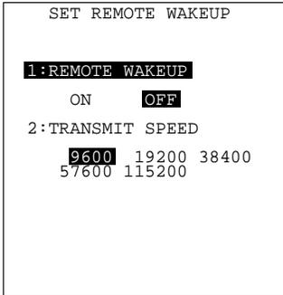
Pressing the **[4]** key while holding down the **[SF]** key on the SYSTEM MENU calls up the screen shown at left.
