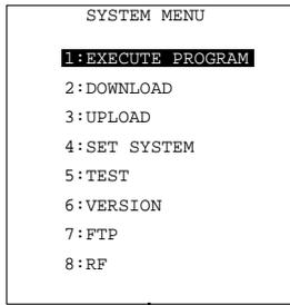
**SYSTEM MENU** ← Press the **PW** key while holding down the **SF** and **1** keys.
