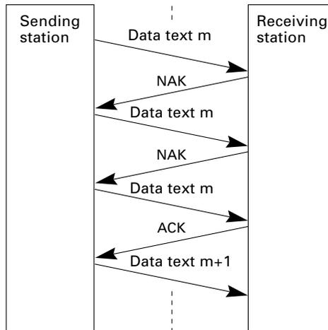
If the sending station receives a NAK 10 times in succession or it fails to send a same transmission block, it shifts to phase 3 to terminate the message transmission abnormally. Even if phase 3 terminates normally, the transmission results in an abnormal end.
