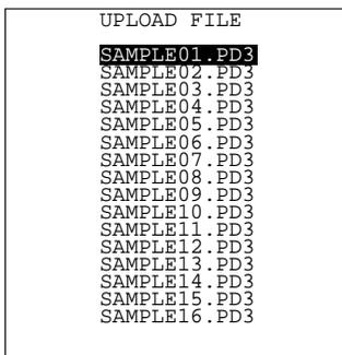
If you select "1:ONE FILE" on the UPLOAD menu, the file selection screen as shown at left will appear, listing all of the program files and data files stored in the memory. Select a file(s) you want to upload and press the key.
