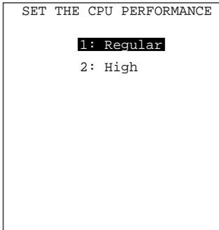
Pressing the **[5]** key while holding down the **[SF]** key on the SYSTEM MENU calls up the screen shown at left.
