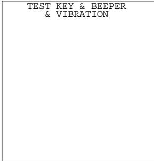
Selecting "7:KEY & VIBRATION" on the TEST menu calls up the screen shown at left and makes the BHT ready for entry from the keypad.
