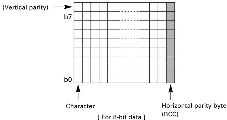
Shown below is a data text block indicating the bits to be added for horizontal parity checking.
