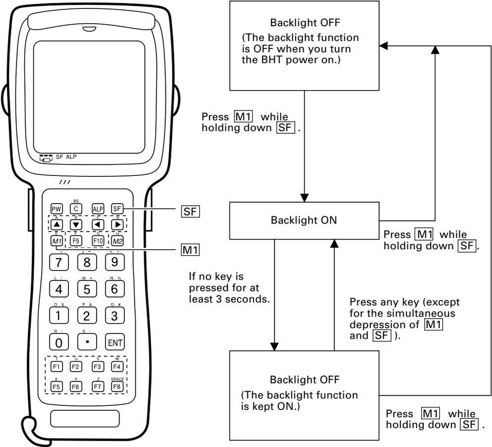
**NOTE** In user programs, you can select the key to be used for activating or deactivating the backlight function (instead of the initial setting: combination of **SF** and **M1**), as well as modifying the ON-duration of the backlight before the automatic turning-off.
