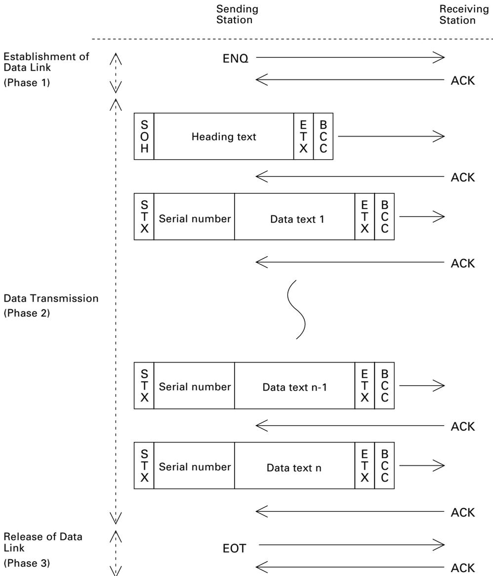
Data transmission may accidentally involve various types of errors. The BHT-protocol is designed to recover from those errors as frequently as possible.
