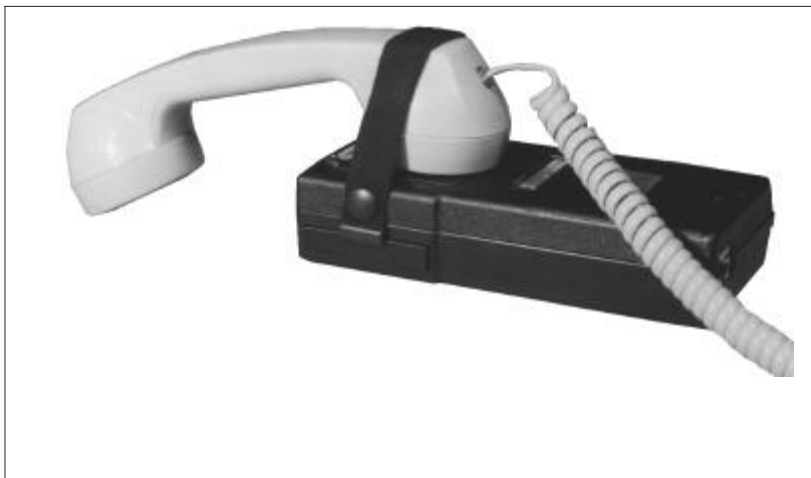
Figure 11. Attaching the Acoustic Coupler to a Receiver
