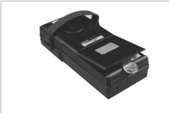
Figure 2. Removing the Battery Compartment Cover
