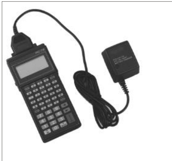
Figure 8. Connecting the Battery Charger
