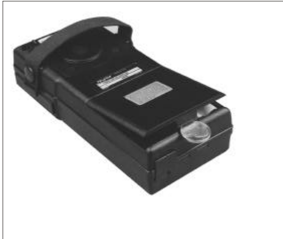
Figure 6. Removing the Battery Compartment Cover
