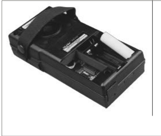
Figure 7. Replacing Alkaline Batteries
